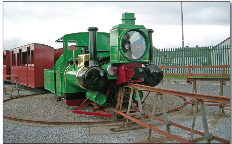
The replica steam outline Listowel & Ballybunion locomotive encounters one of the points. The train travels at 15mph while on the main line, approximately the same speed as the originals.
